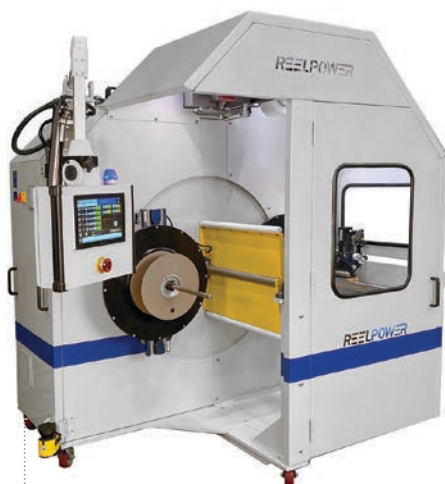
Downstream system for high-speed tubing from Novatec will be furnished with high-capacity coiling/winding equipment from Reel Power.
