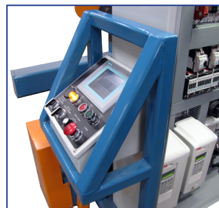
Guarded Control Panel
