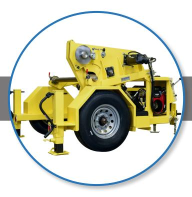
Self-loading powered reel raise and lower
