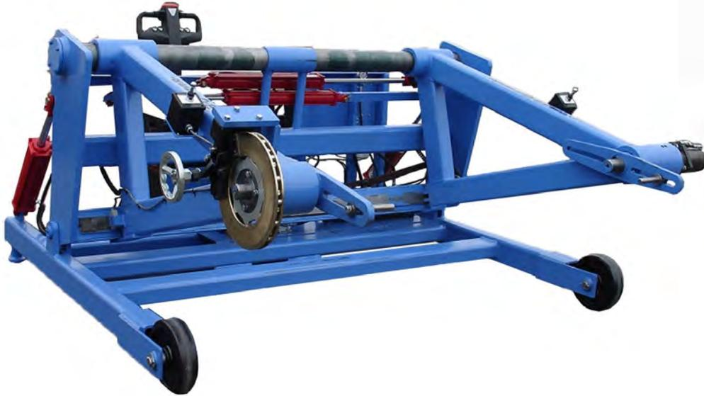
The PRT13 doubles as a High Capacity Payoff System with options including a 16" Bronze Ventilated Disc or Electromagnetic Tension Brake System and Powered Payoff and Rewind Assist Reel Rotation.
