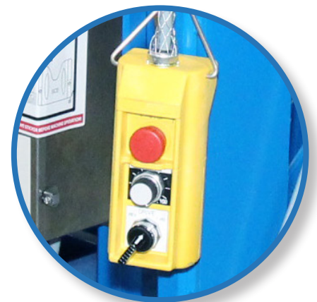
Pendant with Variable Speed Control
